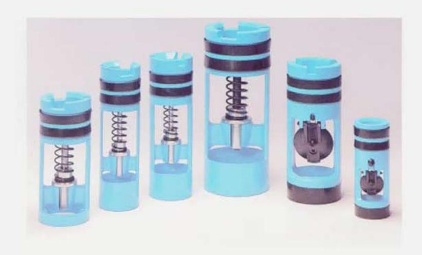
Our Float valves are easy to install. Simply lubricate the side seal rubbers and slide the float valve into the cavity in the float body or drilled out drill collar.
